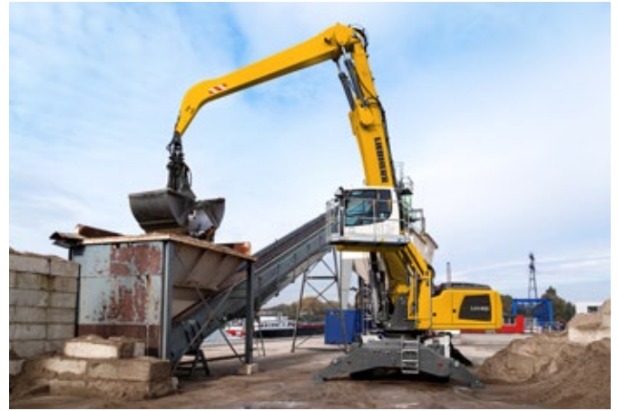
Loading a concrete mixing plant with the LH 40 M Industry Litronic
